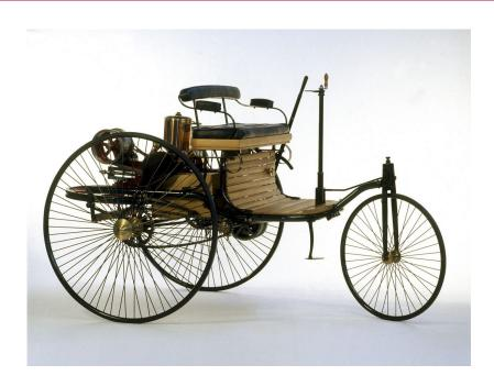
In 1885, German engineer Karl Benz built the world's first automobile powered by an internal combustion engine. The vehicle, called the Benz Patent-Motorwagen, was a three-wheeled machine with an engine capable of producing only two horsepower. Although Benz received a patent for his automobile in 1886, he struggled to find buyers for his machine as he had never tested it over long distances; he had only driven it around his shop in Mannheim.
